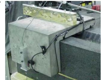
**References:** Vee & Flat bearings used on many common machine tools where gravity provides preload. NEAT uses two magnet tracks, one horizontal and one vertical, to provide horizontal and vertical preload force. Patent search revealed no other relevant art.
